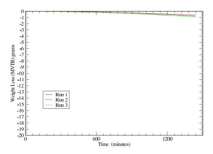
**TABLE 4.** Allevyn Non-Adhesive Moisture Vapour Transmission Rate over 24 hours
