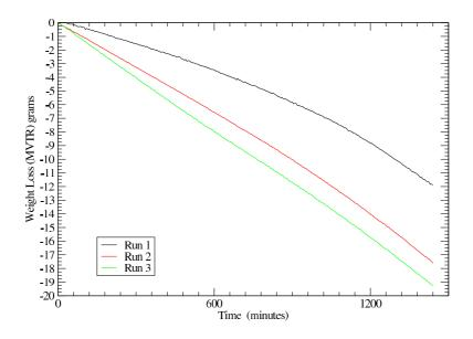
TABLE 5. Versiva XC Non-Adhesive Moisture Vapour Transmission Rate over 24 hours
