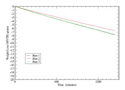
TABLE 3. Versiva XC Adhesive Moisture Vapour Transmission Rate over 24 hours
